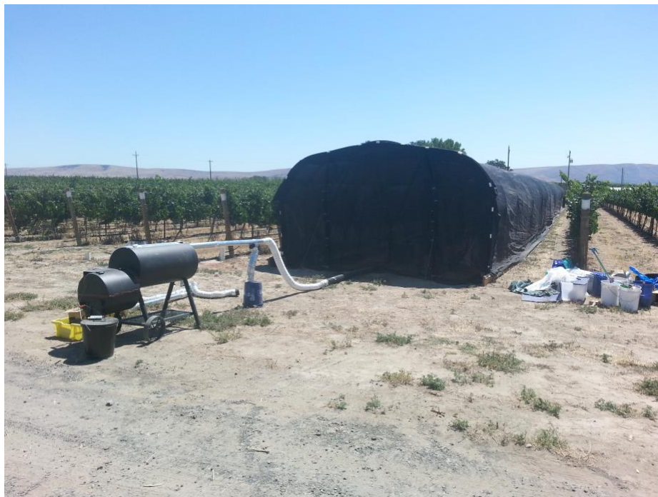
Figure 1. Modular portable hoop-house for conducting controlled smoke exposures
