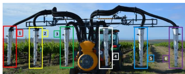
Figure 5: 3-Row Gregoire sprayer equipped with 6 wind socks each with 5 pneumatic nozzles. The angle of the fans should be directed into and slightly behind the canopy with 18-24" between the canopy and nozzle.
