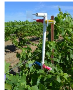
Figure 1: Plastic collection cards in 5 zones per vine and replicated 5 times.
