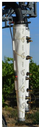
Figure 6: One wind-sock with 5 nozzle bodies that are turned on/off in groups of 3 and 2.
