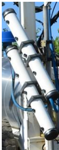
Figure 8: One set of tubes with-10 nozzle bodies that emit charged particles.
