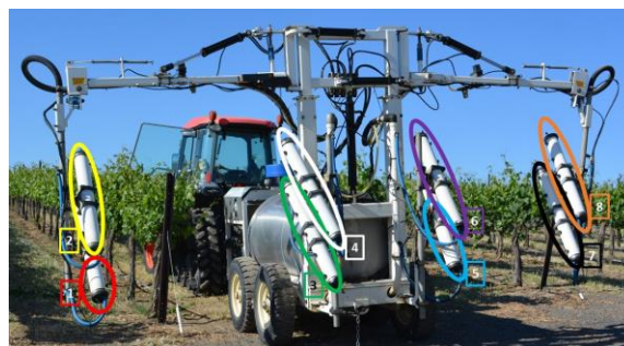
Figure 7: 2-Row On Target Electrostatic sprayer equipped with 8 tubes each with 5 pneumatic nozzles each. The angle of the tubes should be directed into the canopy with 18-24" between the canopy and nozzle.
