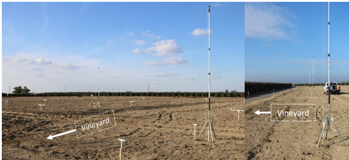
Figure 6. Views of the field setup showing installed horizontal sampling structures and vertical string sampling structures. Photo credits: Peter Larbi.
