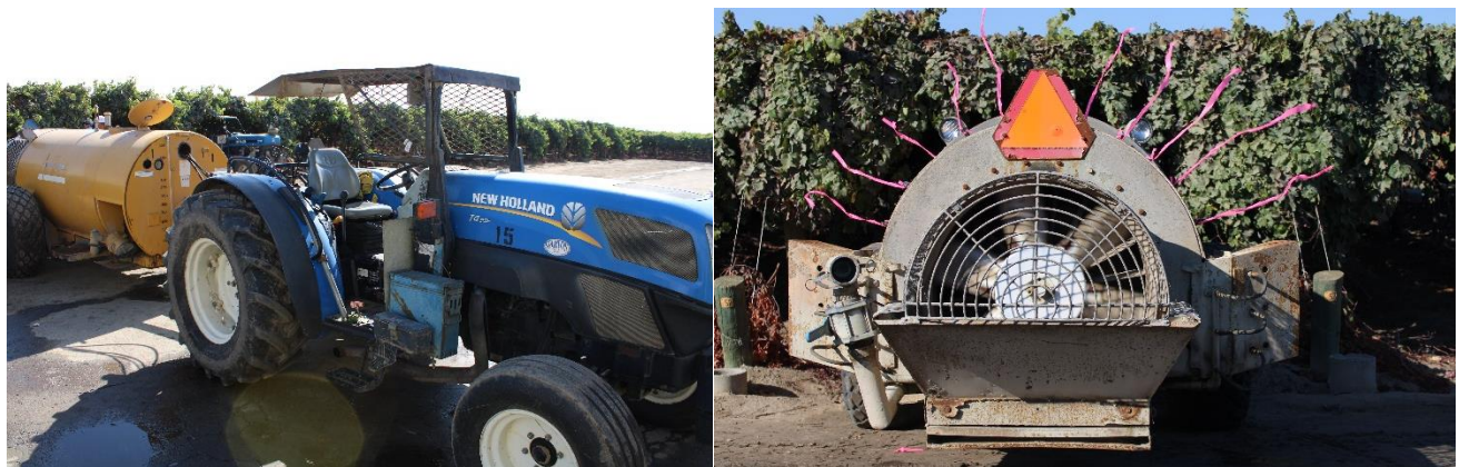
Figure 4. Airblast sprayer used in experiment: left – sprayer-tractor hook-up; right – back view showing air profile depicted with marking tape. Photo credits: Peter Larbi.
