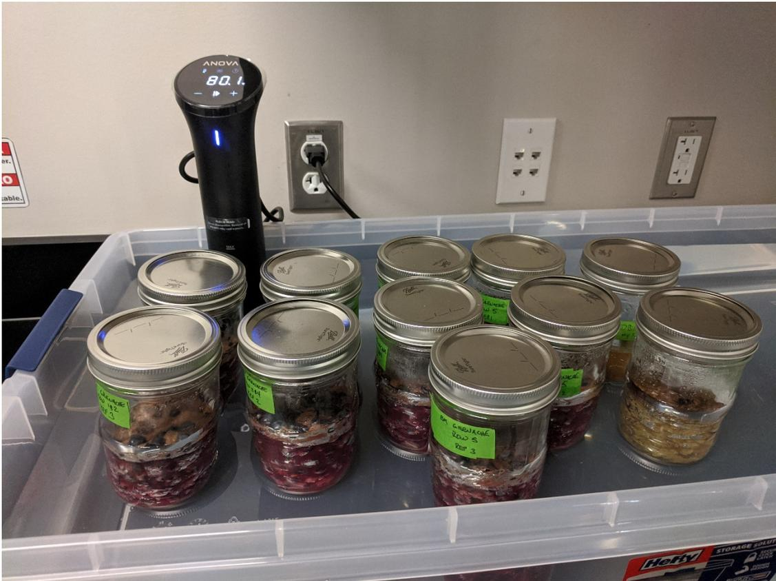
Figure 1 Under-the-bed storage box set up as a nano-scale fermentation water bath, with sous vide machine for temperature control. These are 16 oz. canning jars, with lids and bands loosely applied to allow CO<sub>2</sub> to escape.
